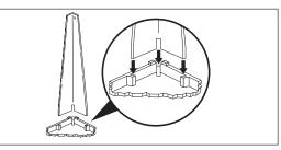
3. Place a block of wood over the end of the leg and drive the leg down into the socket with a hammer.
