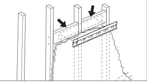
2. Determine the comfortable working height of the top off the sink. This height may vary depending on you application, however, a typical dimension is 32" up from the floor. Use a level to mark a line 1" below the desired height of the wall.
