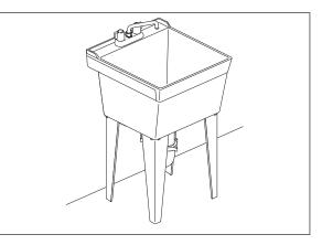
2. On the wall mount models only, lift and place the sink over the wall mounting plate. Make sure the sink is seated securely into the lip of the wall mounting plate.
