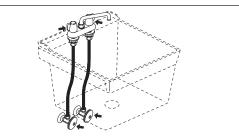
Check all water lines and waste connections for leaks. Tighten the connection if a leak appears. Do not over-tighten.
