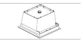
Find the right-side filler bracket. Install it with the end of the filler bracket fitted between the outside of the sink and guide posts. (1). Also place the filler bracket over the guide post (2) and the screw hole in the bottom of the sink / tub.
