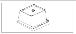
2. Slide the metal or plastic leg onto one of the plastic corner retaining sockets in the bottom of the sink / tub. All legs are identical and can be installed in any one of the four corners.
