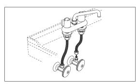
5. The water lines and waste pipes should not be completely installed.
