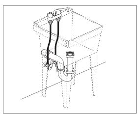
6. Slowly turn ON the hot and cold water shut off valves. Turn the faucets ON and flush the water lines to remove any debris that may be in the water line or drain pipe.
