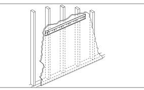
If only two screws can be used, install cross blocking (2" x 6") between the studs and then attach the wall mounting plate. Again, for double sinks install cross blocking (2" x 6") between the studs to add extra support for the wall mounting plate and the sink.
